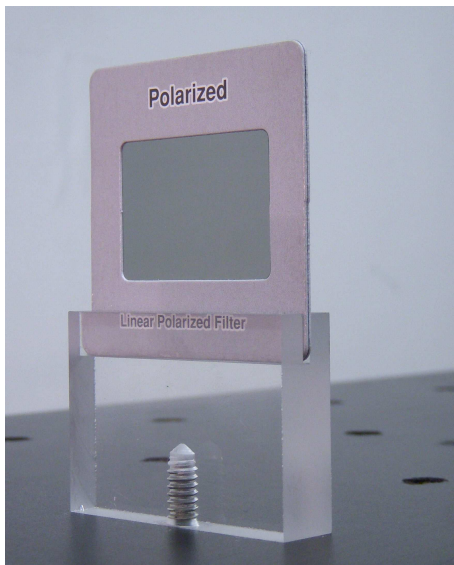
Polarizer mounted in slide holder with acrylic support (LABEL J).
