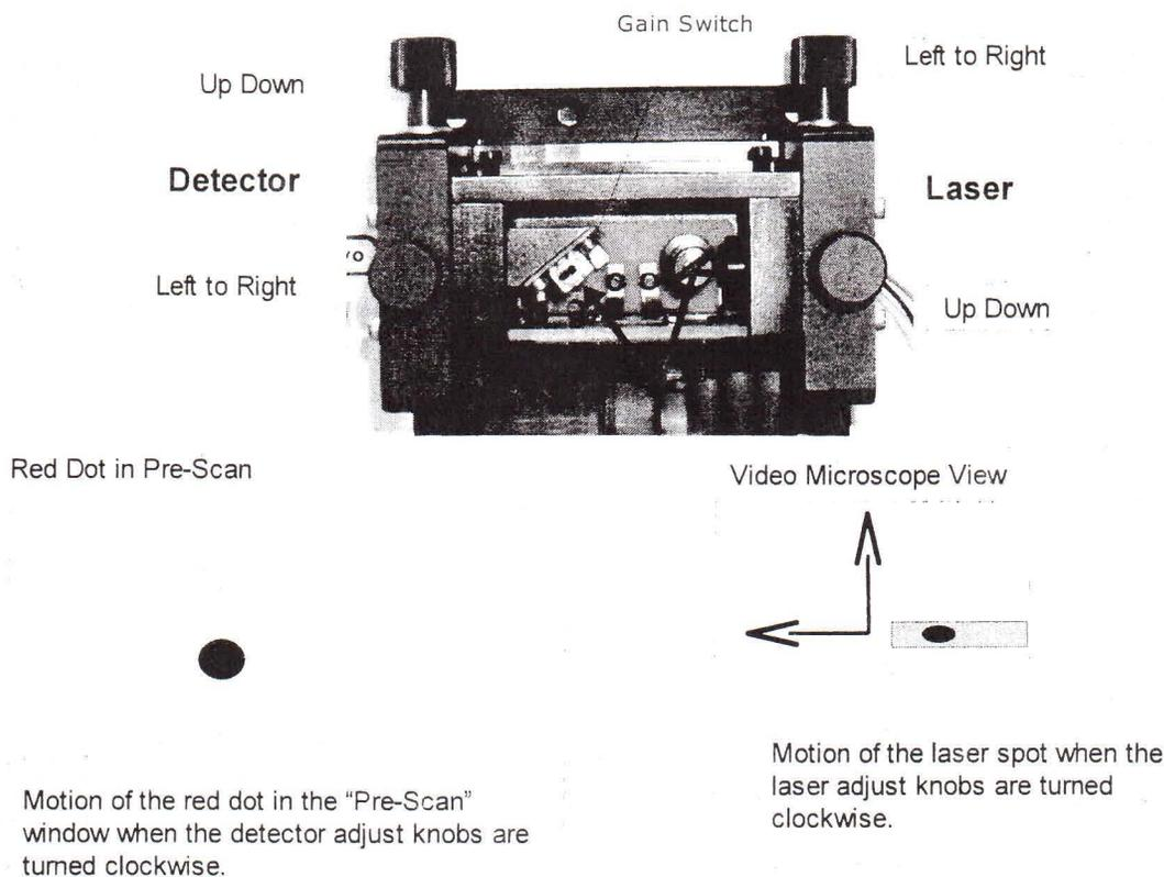
Tips for aligning the laser in the light lever force sensor:
